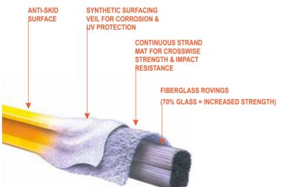
Fiberglass reinforcements (fibers and mat)
